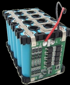
Lithium battery + BMS
