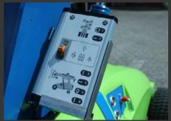
Multifunction control panel in operatorfriendly design with integrated buttons and signal lights. Double action safety keys and Gyro functionality are both in the standard setup on the Winlet 785.
