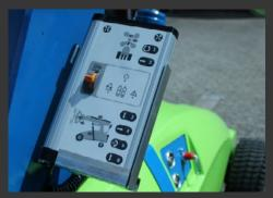
Multifunction control panel in operatorfriendly design with integrated buttons and signal lights, Double action safety keys and Gyro functionality are both in the standard setup on the Winlet 575.
