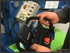
Multifunction control panel in operatorfriendly design with integrated buttons. Signal lights and Double action safety keys are both in the standard setup on the Winlet 350TH.
