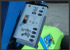
Multifunction control panel in operatorfriendly design with integrated buttons and signal lights, Double action safety keys and Gyro functionality are both in the standard setup on the Winlet 1000.
